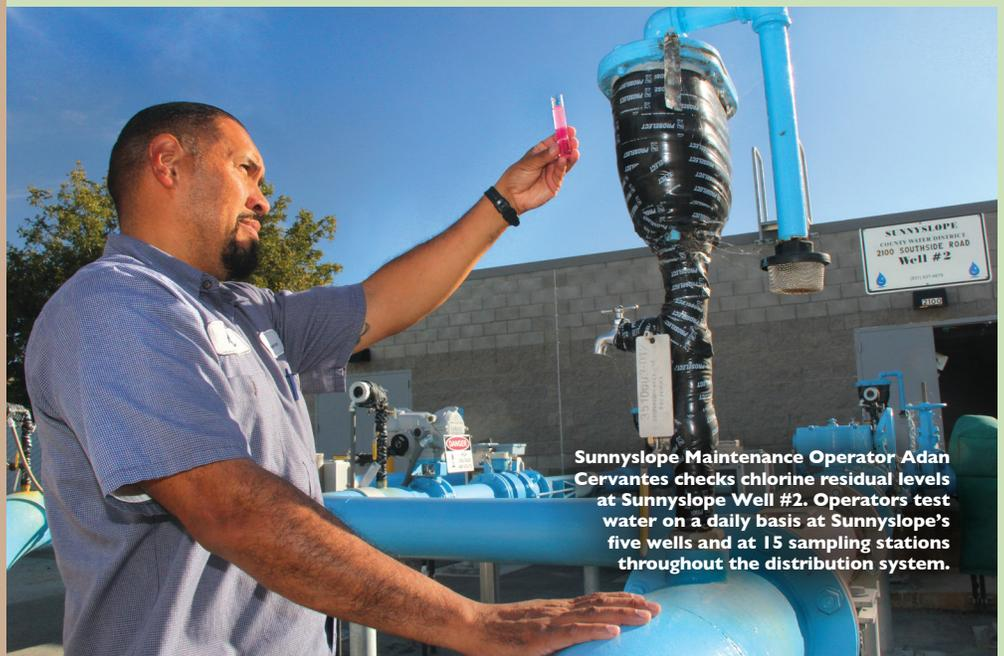
**Sunnyslope Maintenance Operator Adan Cervantes checks chlorine residual levels at Sunnyslope Well #2. Operators test water on a daily basis at Sunnyslope's five wells and at 15 sampling stations throughout the distribution system.**
