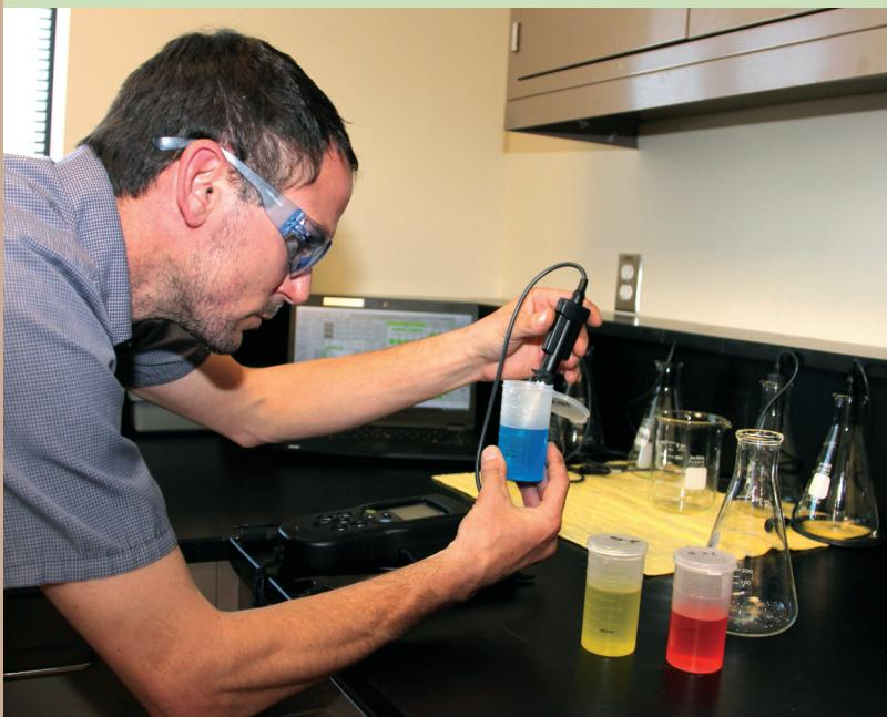
**Water Treatment Operator Troy Quick tests pH levels at the West Hills treatment plant. Sunnyslope personnel continually test water at all stages of the treatment process and throughout our distribution system to ensure the delivery of clean, safe water to our community.**
